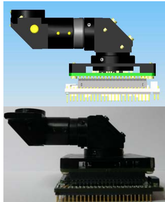
Fig. 6 The Goliat Camera. CAD view (top), real model (bottom)
