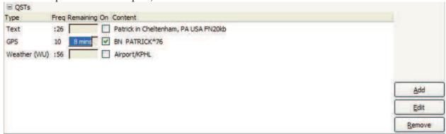
Use the add button to create a new QST. This example shows a temperature report from an airport. Select the type and interval between bulletins from the drop down lists. You may enter the number of minutes directly. Additionally, a colon may be placed before the number to make the time absolute. (:56 = 56 minutes past the hour).
